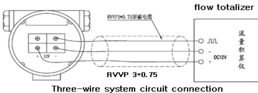
**8.1.1** Main power supply and output signal terminals .( Use the Three-wire shielded cable.RVV P 3\*0.75)
