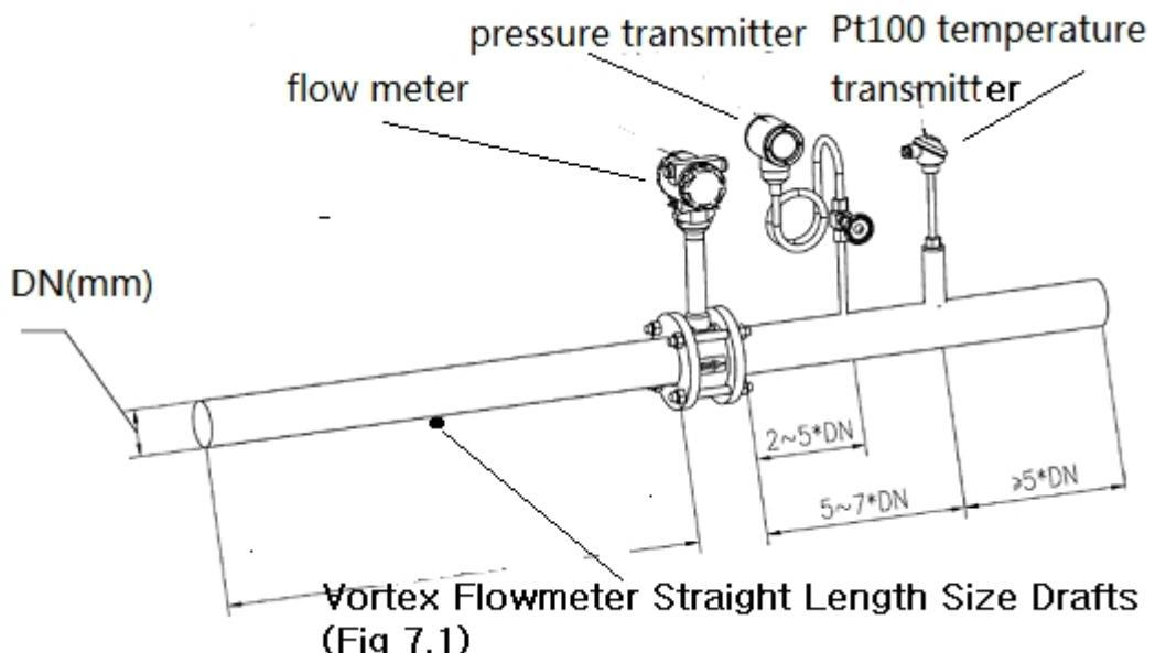
**7.10** After initial installation, when medium is steam or other high-temp medium, flanges & bolts should be re-tightened when medium full of pipeline. Do heat reservation measures for pipeline in order to protect amplifier.
