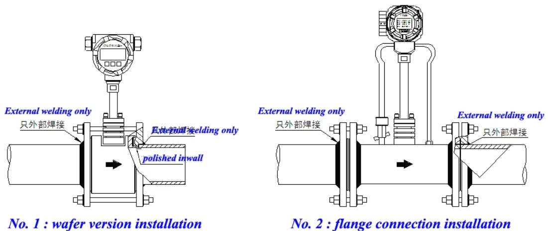
**7.3** use our special gaskets for Vortex diameter, Fit a gaskets inside the groove of the flange.
