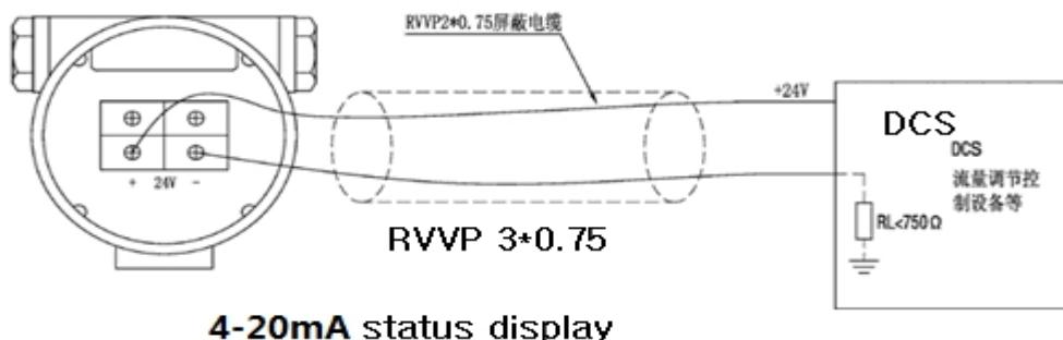
**8.2.1** Main power supply and output signal terminals ( Use the Two-wire shielded cable RV VP 2\*0.75).
